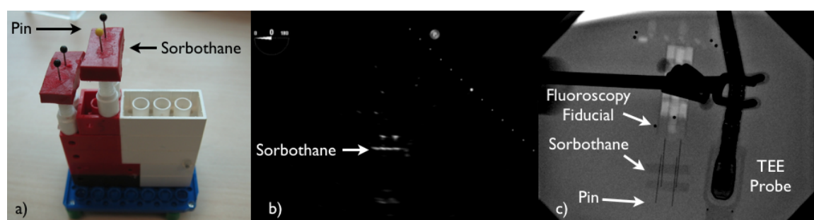
Fig. 4.7: (a) Pin Target Phantom. (b) TEE image of pin target phantom. (c) Fluoroscopy image of pin target phantom.
