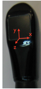
Fig. 3.8: (b) Coordinate system used for relative tracking accuracy study, where the x-y plane lies on the sensor surface.
