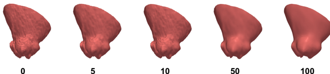
Fig. 6.8: CT meshes used with differing number of smoothing steps in multi-resolution registration.
